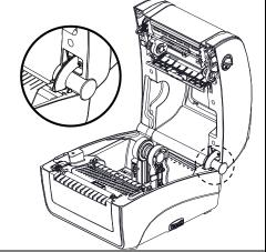
printer will engage with lower inner cover to hold the printer top cover open.
