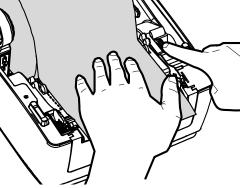
5) Move the media guides to fit the label width by turning the guide adjuster knob.
