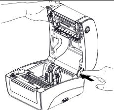
(3) Hold the top cover and press the top cover support to disengage the top cover support with lower inner cover. Gently close the top cover.
