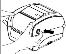
(1) Open the printer's top cover by pulling the top cover open levers located on each side of the printer and lifting the top cover to the maximum open angle.
