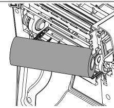
(3) Insert the ribbon right side onto the supply hub. Align the notches on the left side and mount onto the spokes.
