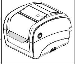
(6) Disengage the top cover support and close the top cover gently.
