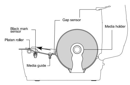
(7) Use "Diagnostic Tool" to set the media sensor type and calibrate the selected sensor. (Start the "Diagnostic tool" → Select the "Printer Configuration" tab → Click the "Calibrate Sensor" button ) Please refer to the diagnostic utility quick start guide for more information.
