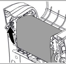
(5) Turn the ribbon rewind gear until the ribbon plastic leader is thoroughly wound and the black section of the ribbon covers the print head. Close the ribbon access cover and the top cover.
