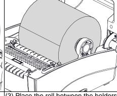
side towards the front of the printer, then lift the top cover to the maximum open angle.
