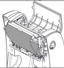
(4) Stick the ribbon onto the ribbon rewind paper core and insert the paper core onto the rewind hub.
