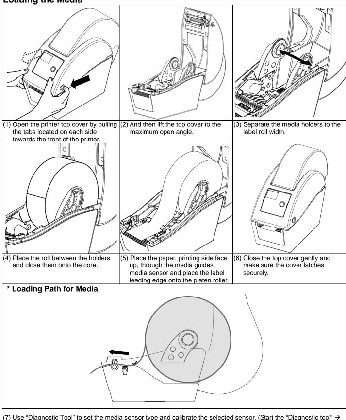
(7) Use "Diagnostic Tool" to set the media sensor type and calibrate the selected sensor. (Start the "Diagnostic tool" → Select the "Printer Configuration" tab → Click the "Calibrate Sensor" button )
