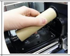
(3) Insert the left side first. Mount the ribbon rewind paper core on the front hubs. Please be noted that the bigger hub side with 4 ribs must be installed toward the right side of ribbon mechanism.
