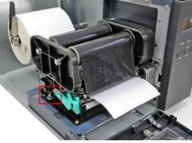
(5) Engage the printer carriage. Select the using label type by sensor switch.
