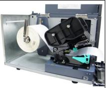
(3) Install the label so that it goes (when using an external label roll mount: through the label feed slot) in the direction of the LABEL label and under the ribbon mechanism to lay upon the platen.
