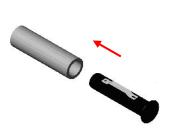
(2) Place an empty paper core onto the ribbon rewind spindle.
