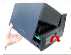
(1) Open the printer cover, front panel and print head release lever.
