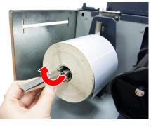
(2) Lower the label roll guard to the horizontal position, slide the label roll into onto the (external) label supply spindly, and then flip back the label roll quard.
