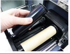
(4) Insert the left side first. Install a ribbon on the ribbon supply spindle. Mount the ribbon supply spindle on the rear hubs.
