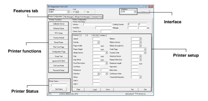
(3) The detail functions in the Printer Function Group are listed as below.
