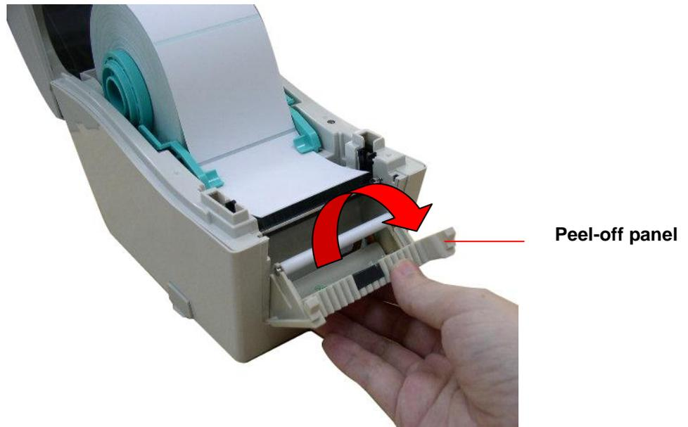
3. Lead the media through the backing paper opening, beneath the peel-off roller.
