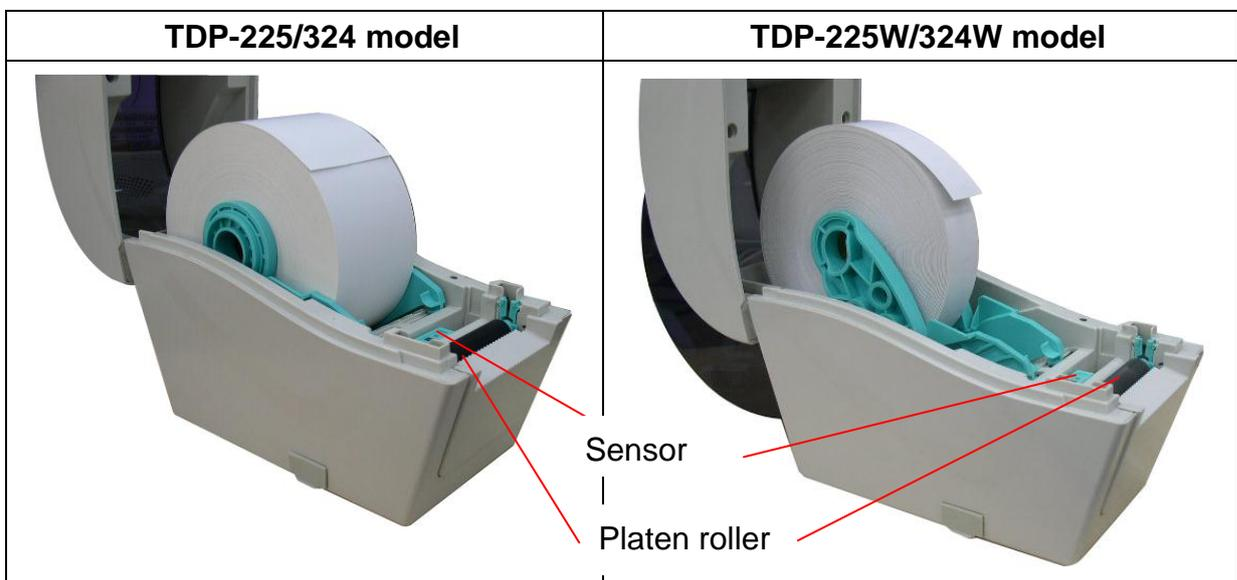
5. Place the paper, printing side face up, through the media guides, media sensor and place the label leading edge onto the platen roller.
