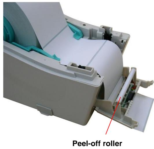
4. Push the peel-off panel back to the printer.
