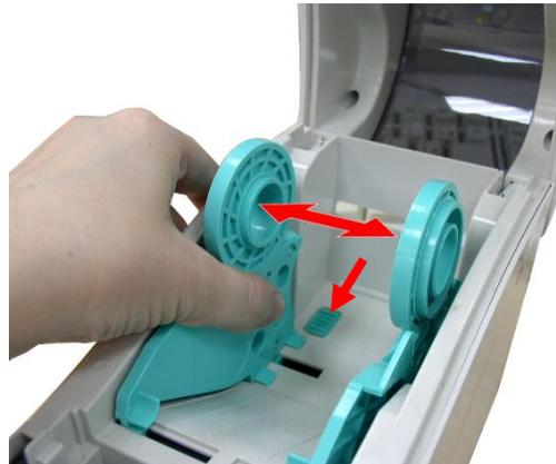
3. Feeds the media through the rear external label entrance chute. And place the paper, printing side face up, through the media guides, media sensor and place the label leading edge onto the platen roller.
