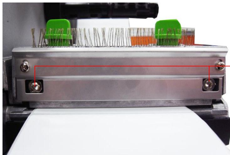
Print head burn line adjustment knobs
