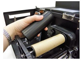
5. Please be noted that the bigger hub side with 4 ribs must be installed toward the right side of ribbon mechanism.
