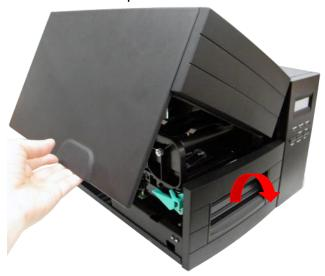
2. Lower the label roll guard to the horizontal position, slide the label stock into label roll spindle, and then flip back the label roll guard.
