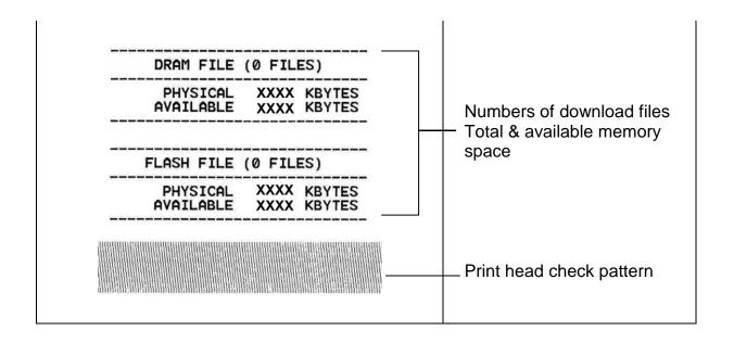
When the self test is completed, the printer enters the dump mode. Please turn the printer's power off and then on again to resume normal printing.
