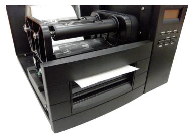
10. Use "Diagnostic Tool" to set the media sensor type and calibrate the selected sensor. (Start the "Diagnostic tool" → Select the "Printer Configuration" tab → Click the "Calibrate Sensor" button) Please refer to the section 4.
