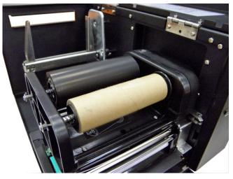
6. Disengage the printer carriage by pulling the print head release lever.
