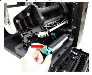
7. Following the direction of the \$\dpres\$ RIBBON label, pull the ribbon leader to the front from beneath the printer carriage.
