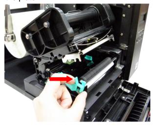
4. Install the label so that it goes (when using an external label roll mount: through the label feed slot) in the direction of the ↓ LABEL label and under the ribbon mechanism to lay upon the platen.
