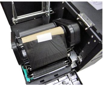
5. Rotate the ribbon rewind roller until the ribbon overlaps the ribbon leader and stretches tight.
