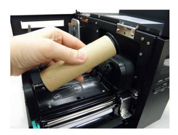
4. Install a ribbon on the ribbon supply spindle. Mount the ribbon supply spindle on the rear hubs. Insert the left side first.
