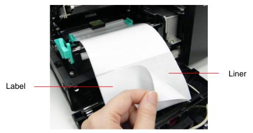
3. Pull the print head release lever to feed the liner between the platen and the white peel-off roller.
