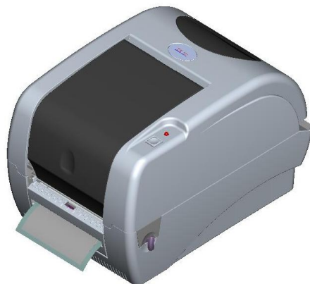
Fig. 21 Complete label installation for peel-off mode
