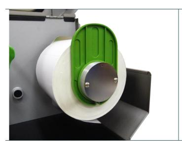
Place the roll of media on the label supply spindle and push it to the end of label spindle. Install the label roll guard gently to fit the width of label roll.
