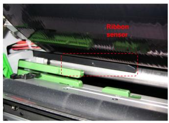
4. Thread the ribbon through the ribbon sensor slot and then through the open space in between print head and platen.
