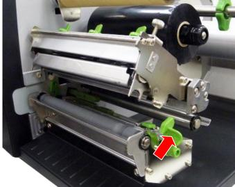
3. Push the print head release lever to open the print head mechanism.
