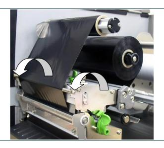
7. Close the print head mechanism making sure the latches are engaged securely.
