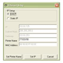
The default IP address is obtained by DHCP. To change the setting to static IP address, click "Static IP" radio button then enter the IP address, subnet mask and gateway. Click "Set IP" to take effect the settings.
