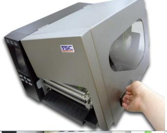
1. Lift the handle to open the printer right side cover.
