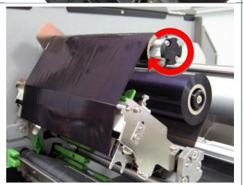
6. Wind the ribbon clockwise about 3~5 circles onto the ribbon rewind spindle until it is smooth and properly stretched.
