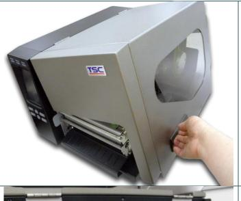
1. Lift the handle to open the printer right side cover.
