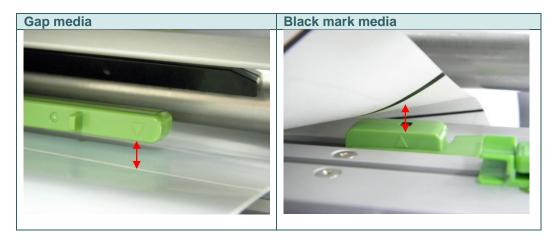
6. Adjust the front label guide to fit the width of the label.
