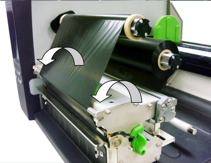
6. Close the print head mechanism making sure the latches are engaged securely.
