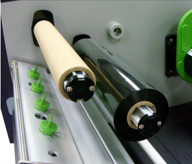
2. Install the ribbon and paper core onto the ribbon supply spindle and ribbon rewind spindle. **Make sure the ribbon & paper core are set at the center of the spindle.** (You can refer to the ruler on the spindles.)
