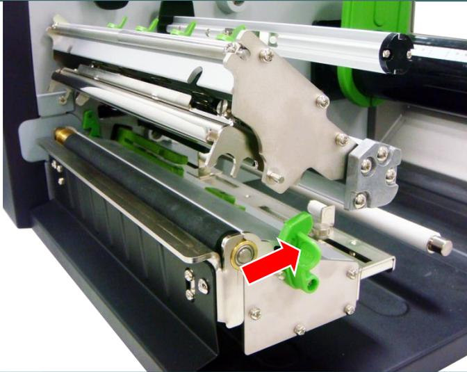
1. Lift the handle to open the printer right side cover. Push the print head release lever to open the print head mechanism.
