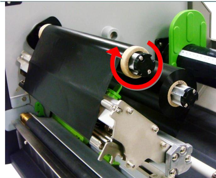
4. Stick the ribbon onto the paper core. Keep the ribbon flat and without wrinkle.
