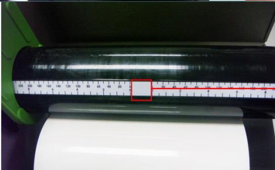
3. Make sure the width of the label. (You can refer to the ruler on the spindles.)
