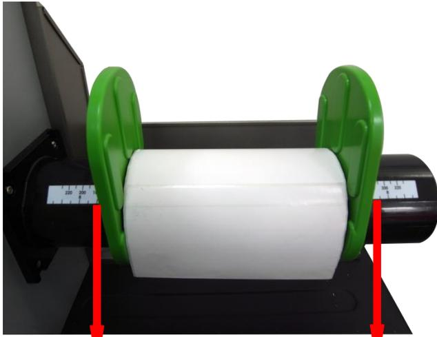
4. Place media roll on label supply spindle. Replace label roll guard. Make sure the label roll guard position of each sides are the same as the length of the label. Please check the outside edge scales are both close to the label width.
