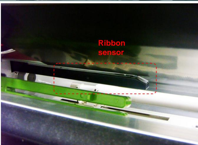
3. Thread the ribbon through the ribbon sensor slot and then through the open space in between print head and platen.
