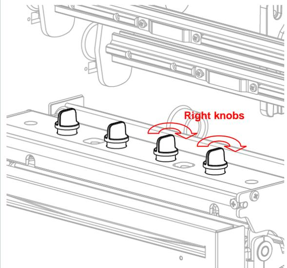
The print head pressure adjustment knob has 5 levels of settings. Clockwise direction adjustment is to increase the print head pressure. Counter Clockwise adjustment can decrease the print head pressure.
