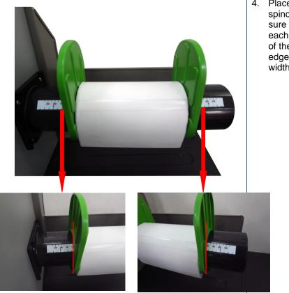
Place media roll on label supply spindle. Replace label roll guard. Make sure the label roll guard position of each sides are the same as the length of the label. Please check the outside edge scales are both close to the label width.
