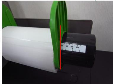
5. Pull label roll leading edge forward through the media guide bar, media sensor (green) and place the label leading edge onto the platen roller.
